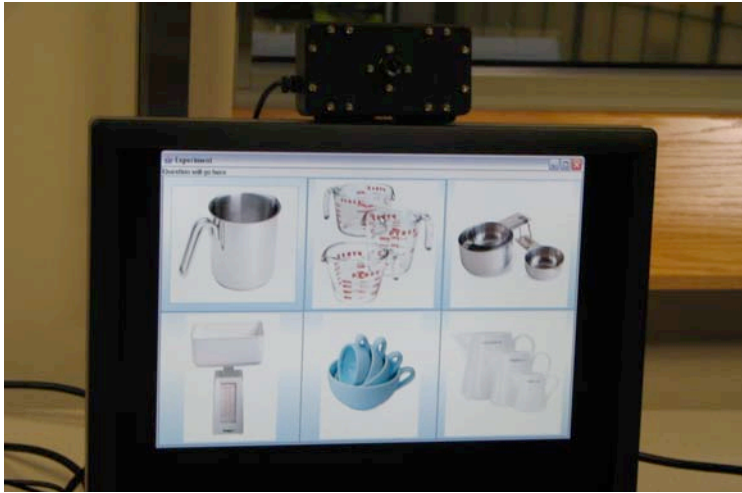
Figure 5. On top of the monitor where the cooking tools are displayed, a small, eye contact sensor was mounted to detect whether the participant is looking in the direction of the monitor (from Torrey et al., 2007).
