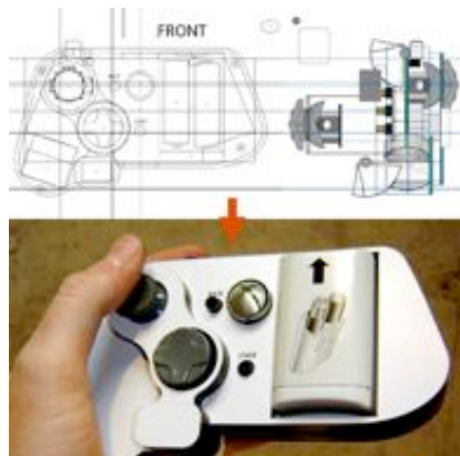
A one-handed Xbox controller—from schematic to built artifact. (Photo credit: Ben Heck)
